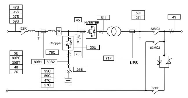
Figure 19 - Protective Detector Locations.
